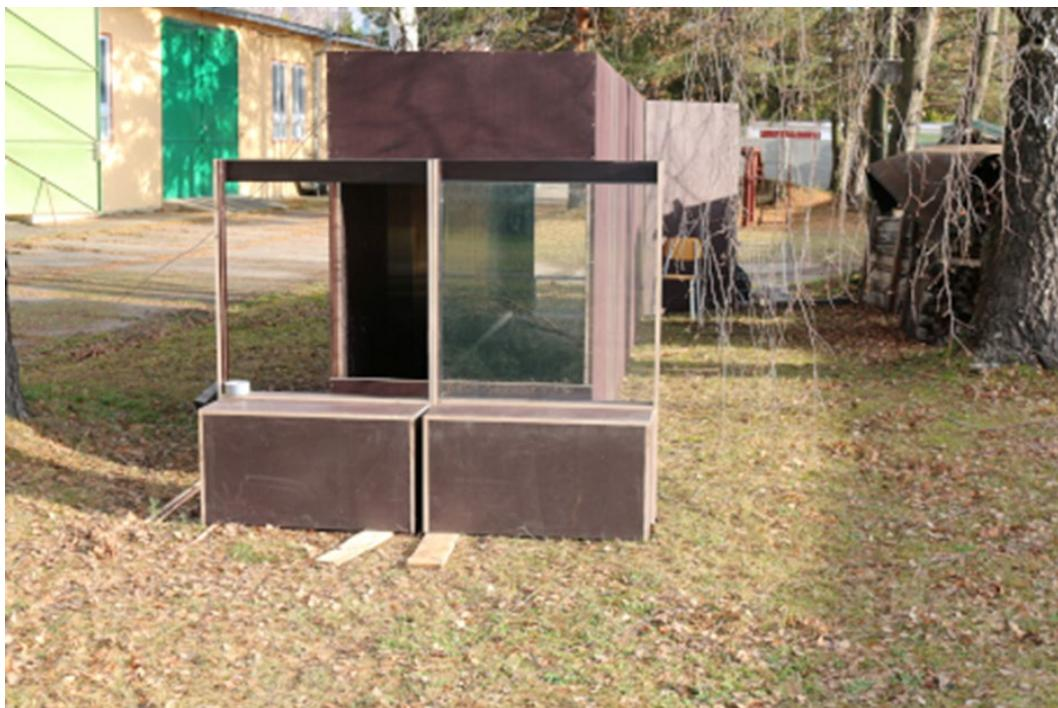
**Figure 2** Escape routes from the test tunnel, left clear glass without laser treatment (Float type clear 4 mm), right surface treated glass (Float type clear 4 mm, dot pitch 1.25 mm at 100% laser power).
