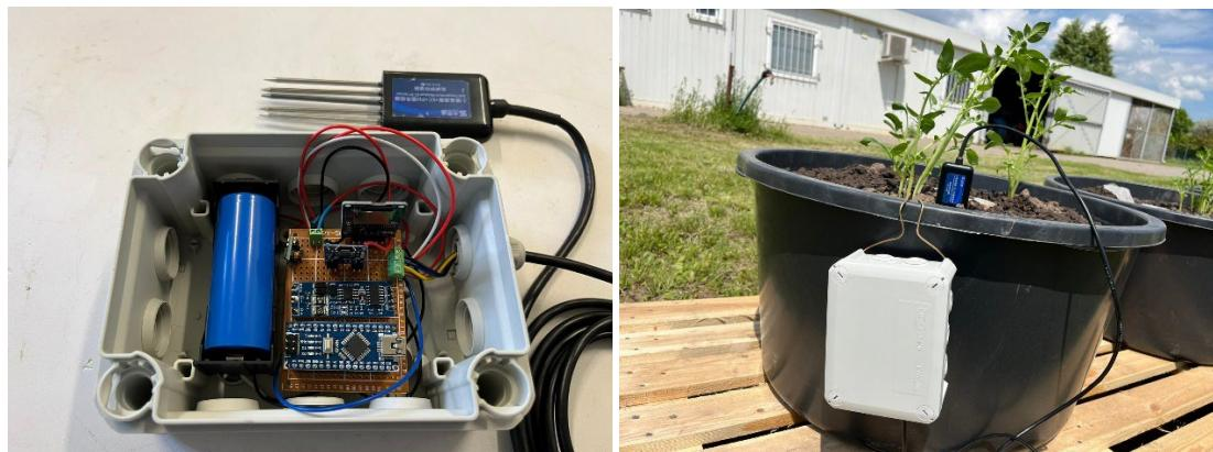
**Figure 2** Data acquisition device with the sensing module and backup and relay modules merged. One the left image is the inside of the device with the battery on the left and Arduino Nano board, micro-SD card module, solar charger module, RS485 to UART bridge and regulator on the right. On the right image is the DAQ with a connected soils sensor automatically collecting data and saving it on an micro-SD card.
