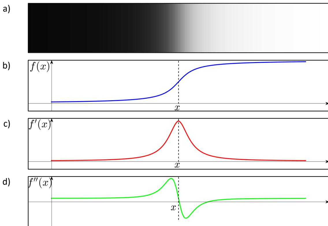
**Figure 1** a) Illustration of the brightness transition, b) representation of the image function of the brightness transition, c) first derivative of the image function, d) second derivative of the image function
