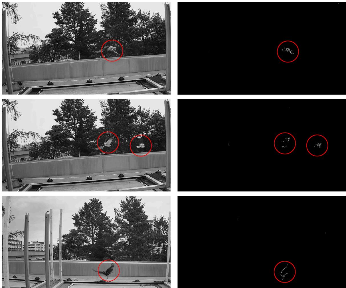
**Figure 3** Identification of birds by detecting changes in the image
