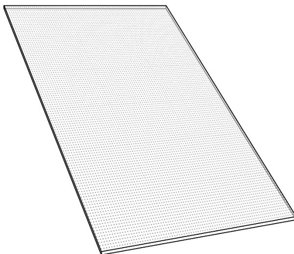
**Figure 1** Visualisation of the print form of the surface treated glass (Float clear 4 mm, dot pitch 1.25 mm at 100% laser power).
