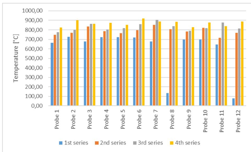
**Figure 3** Visualisation of the values measured by the probes in the computer simulation of the firing of points in individual rows in variant 2
