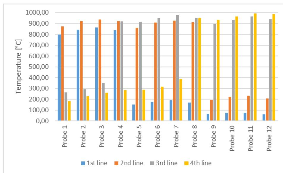
**Figure 2** Visualisation of the values measured by the probes in the computer simulation of the firing of points in individual rows in variant 1
