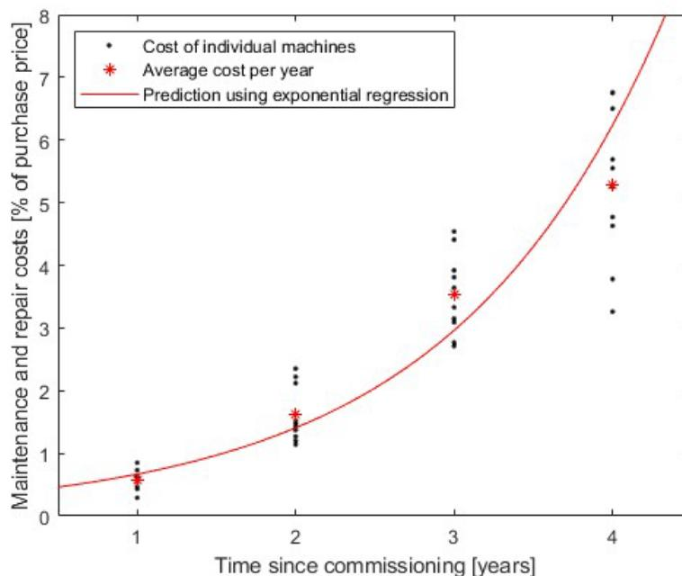
**Figure 3** Predicting tractor repair and maintenance costs using exponential regression
