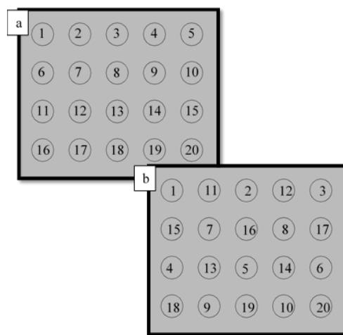
**Figure 1** Order of firing points by laser engraving machine in a) variant 1, b) variant 2
