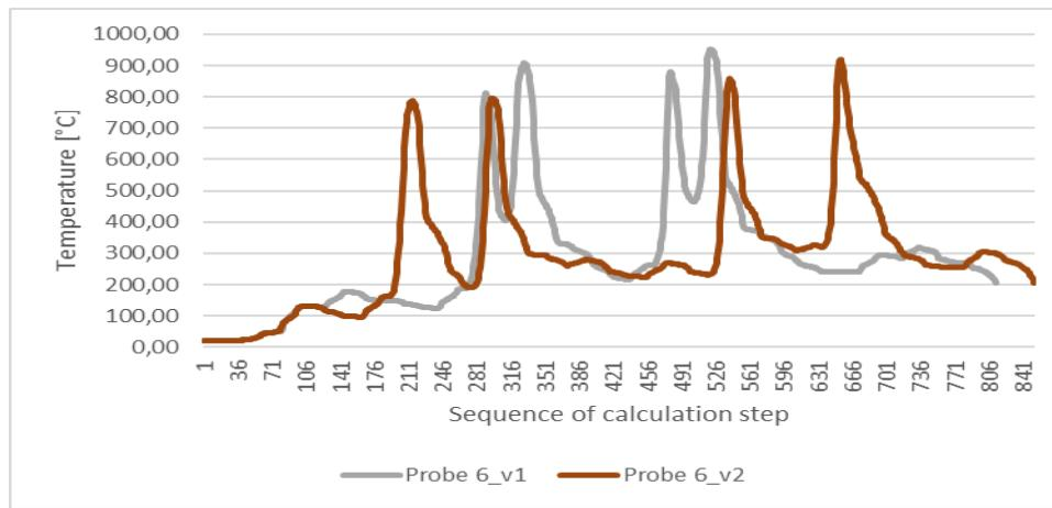
**Figure 5** Comparison of the temperature evolution obtained from probe 6 in the computer simulation of the laser engraving process for Variant 1 and Variant 2.
