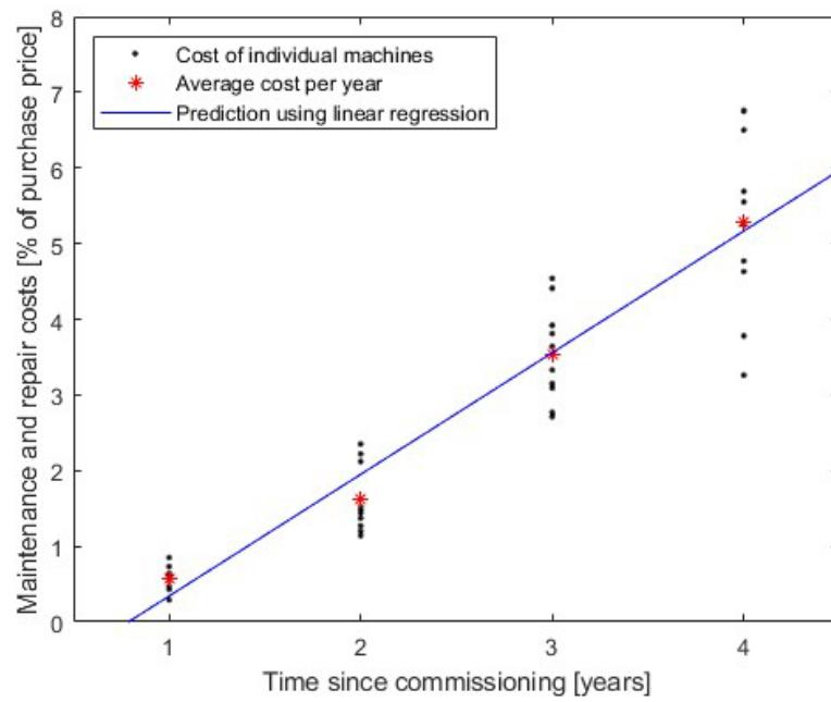
**Figure 4** Predicting tractor repair and maintenance costs using linear regression
