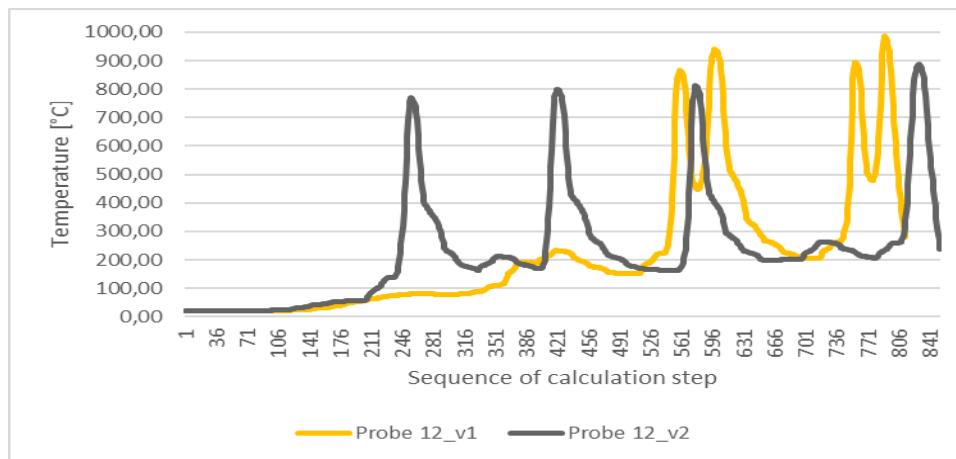
**Figure 6** Comparison of the temperature evolution obtained from probe 12 in the computer simulation of the laser engraving process for Variant 1 and Variant 2.
