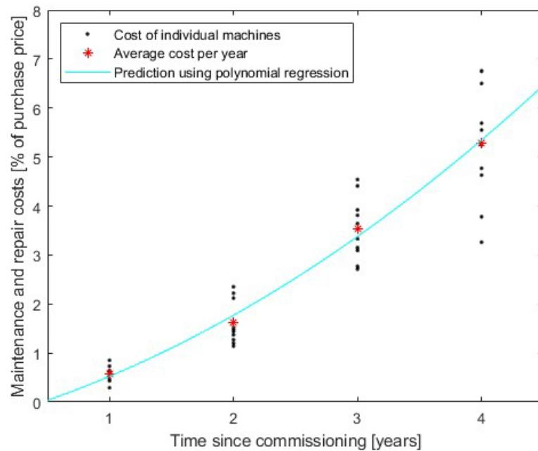
**Figure 5** Predicting tractor repair and maintenance costs using polynomial regression
