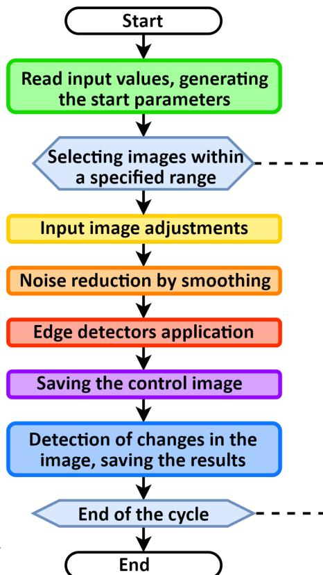
**Figure 2** Basic scheme of the algorithm for detecting changes in the image
