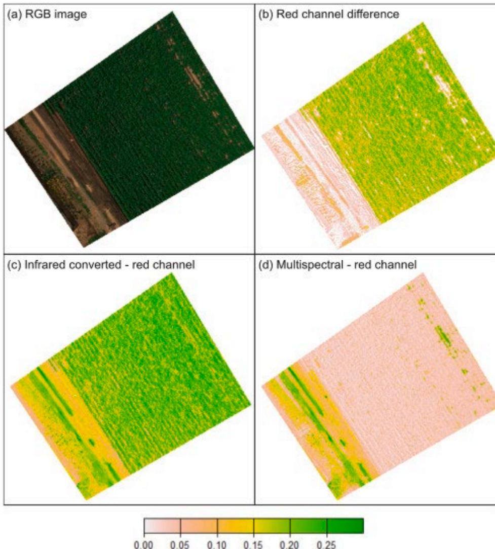
**Figure 2** The difference in red reflectance captured by the infrared converted and multispectral camera for a scene over the potato field. Sub-figure (a) shows a true color (RGB) image, (c) and (d), the red-channel's reflectance from the infrared converted and multispectral cameras respectively, and sub-figure (b) the difference between the two sensor's red-channels. (i.e., infrared converted minus multispectral). (Louw and Chen, 2024)
