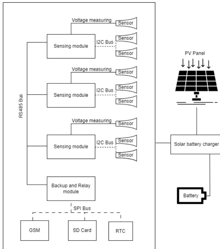
**Figure 1** System Architecture comprising of the three sensing modules that collect data from sensors and send it to the backup and relay module which saves a backup on an SD card in case of connection outage and sends the timestamped data over the GSM on a server over the internet. The whole system is powered by a solar panel charged battery located in a separate container.
