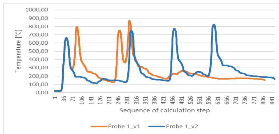
**Figure 4** Comparison of the temperature evolution obtained from probe 1 in the computer simulation of the laser engraving process for Variant 1 and Variant 2.
