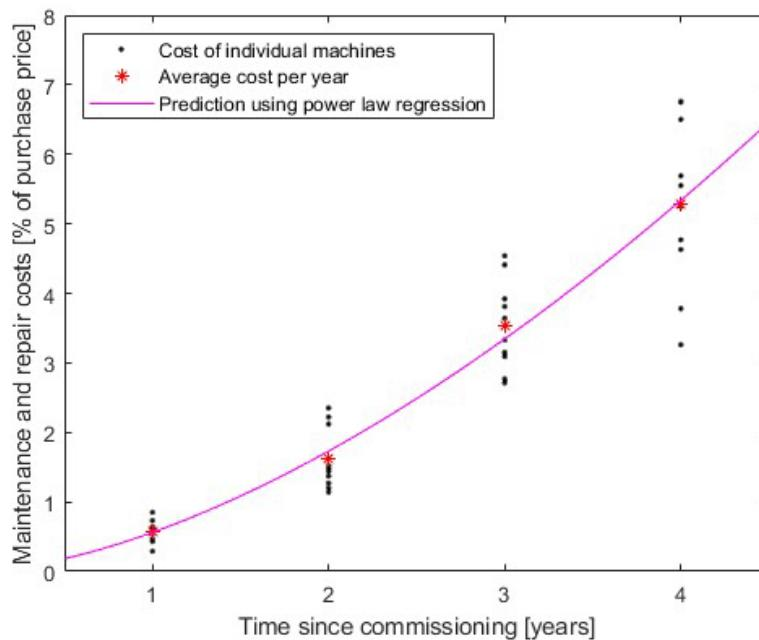
**Figure 6** Predicting tractor repair and maintenance costs using power law regression
