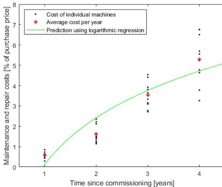
**Figure 2** Predicting tractor repair and maintenance costs using logarithmic regression
