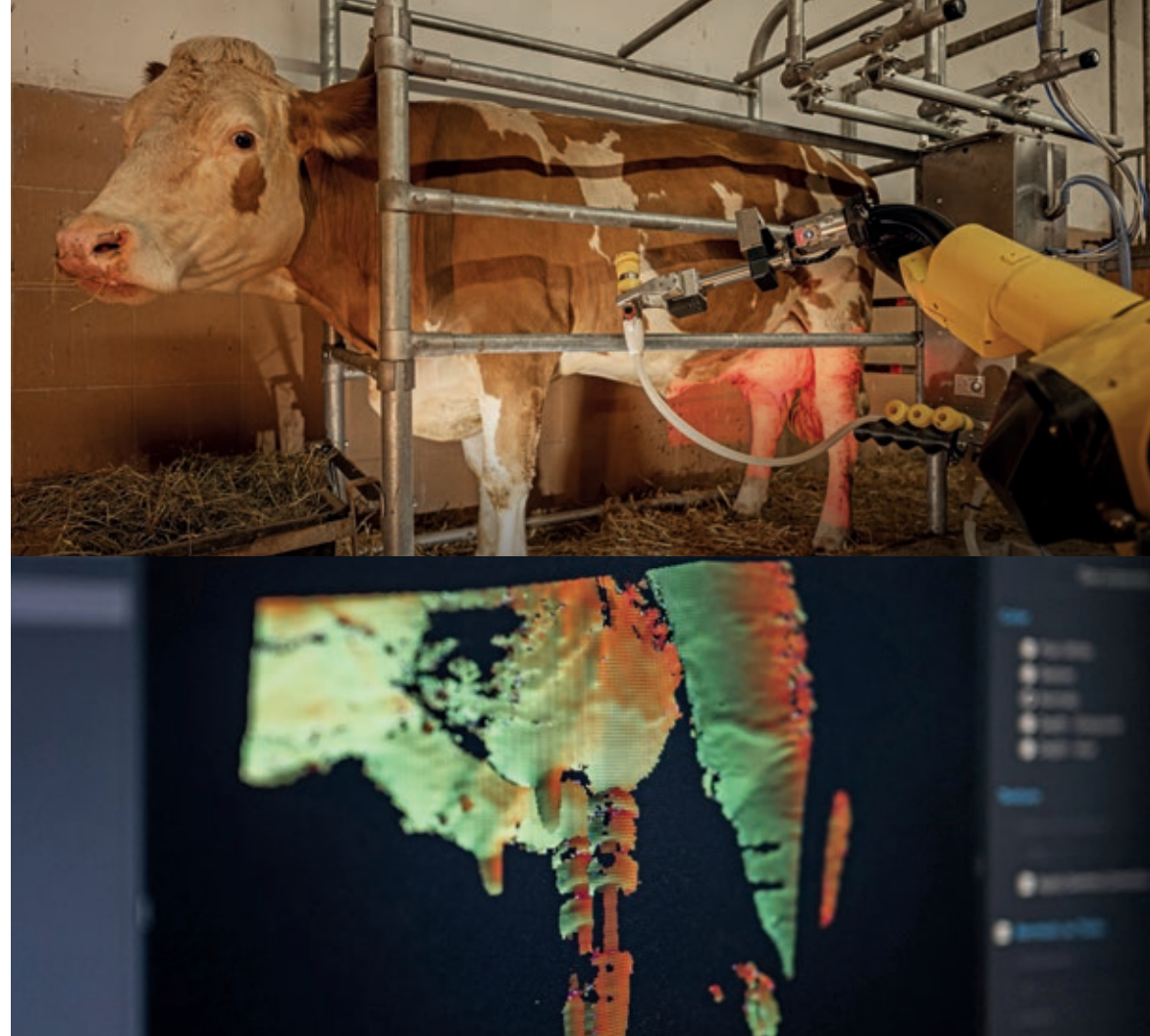
Application of a robotic arm for milking and 3D visualisation of the udder area.
